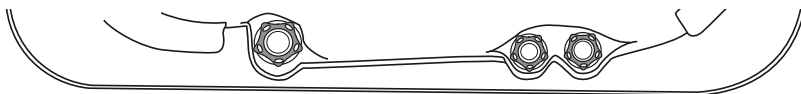
A Mini Diverter Valve, an Air Control, and a Water Diverter Valve. Locations will vary on each spa model.
